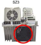
If you find a clogged or defective fan they can be replaced. **We only recommend experienced engineers or technicians attempt repairs on our drives due to safety concerns.** If you would like, a certified CT Technician can repair the drive for you. Contact 1-800-367-8067 and ask for Repairs or Technical Support.
